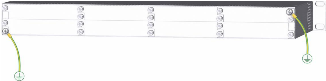
Figure 5: Grounding of the system
