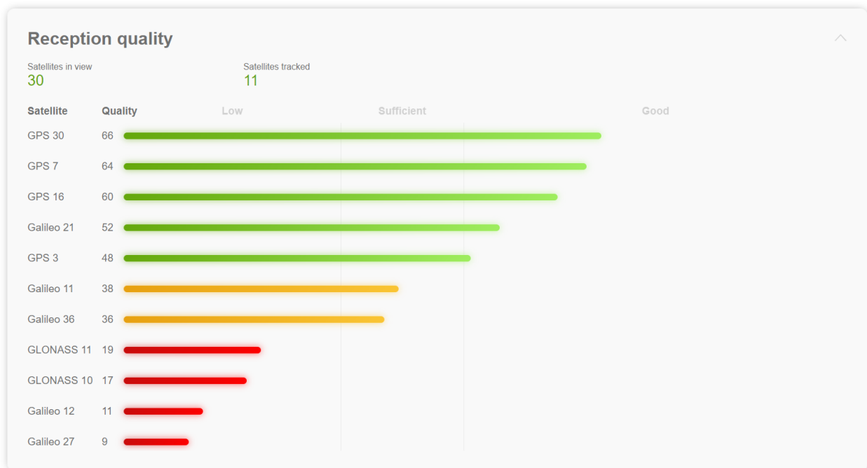
Figure 66 Example of the GNSS reception quality status section
